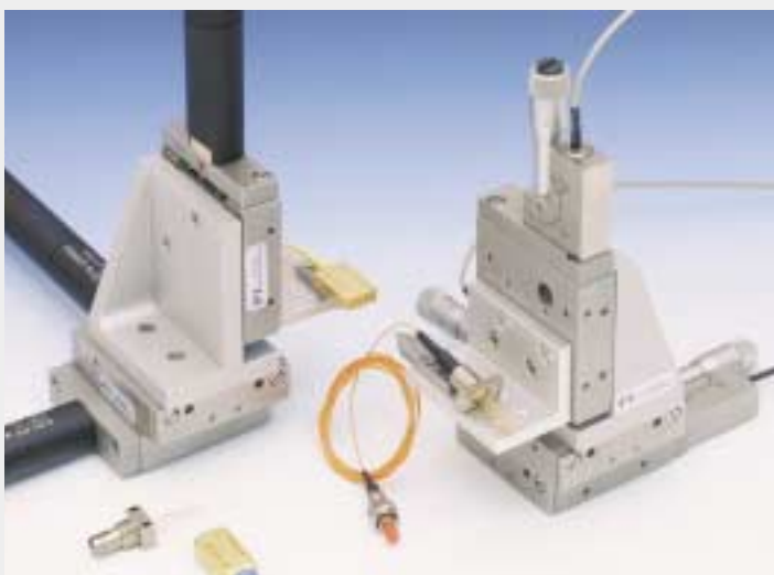
Example of F-110-related photonics alignment systems. XYZ unit on left consists of an M-105.3BA XYZ translation stage with three M-231 DC Mike Drive upgrades and M-009.20 mounting bracket with F-010 V-groove fiber holder. XYZ unit on right consists of an M-105.3BA XYZ translation stage with three P-854 PiezoMike™ upgrades and M-009.20 mounting bracket with F-010 V-groove fiber holder
