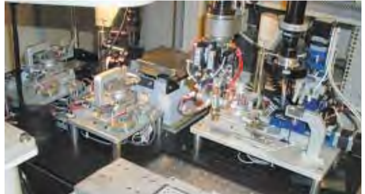
F-206 HexAlign 6-DOF MicroMotion robot deployed as a photonics alignment sub-system for automated assembly of fiber pigtailed devices. Courtesy Aries Innovations
