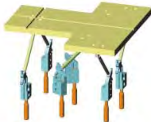
Parallel kinematics of constant-strut-length Hexapod system shows how little mass (basically only the top platform) has to be supported and moved by the six drives. This explains why the F-206 is considerably faster in terms of step-and-settle than standard "stacked" multi-axis systems, where each stage has to support and move it's own platform and the mass of any other stages above it. Also, note that, unlike serial kinematics systems, there are no moving cables to cause friction, tension or torsion to limit accuracy and repeatability.
