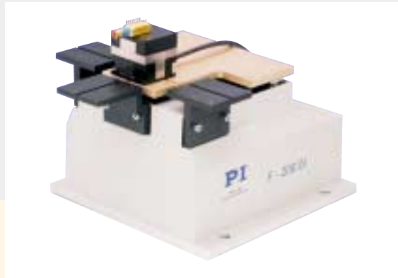
F-206 HexAlign™ 6D alignment system integrates long-travel, high-precision, six-degree-of-freedom motion and linear/rotary alignment automation. Optional high-speed, 100 x 100 x 100 μm, XYZ PZT alignment module achieves nanometer resolution.
