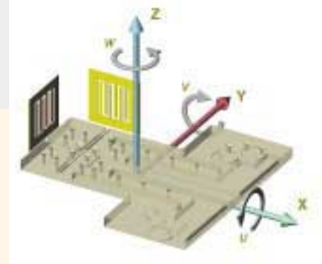
F-206 HexAlign™ Hexapod principle allows motion of platform in all six degrees of freedom. Ideal for angular scans and alignment tasks like those required in collimator packaging applications .
