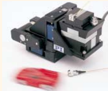
F-130 XYZ rapid-alignment system features 1 nm piezoelectric resolution and 15 mm motorized travel-range in each axis.
