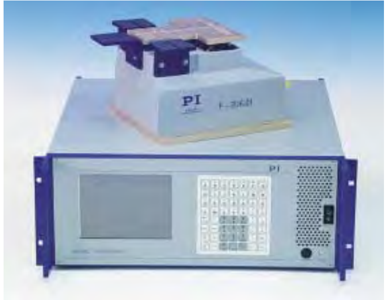
F-206 HexAlign™ System with Digital Controller (figure shows model F-206.00D with display and keyboard). PI's Hexapod controllers perform sophisticated six-space coordinate transformations and path planning internally, automatically. This makes the systems very easy to use, as the unit speaks in terms of familiar X, Y, Z, \theta_x , \theta_y , \theta_z coordinates with millimeter and degree units (4-decimal-place precision).
