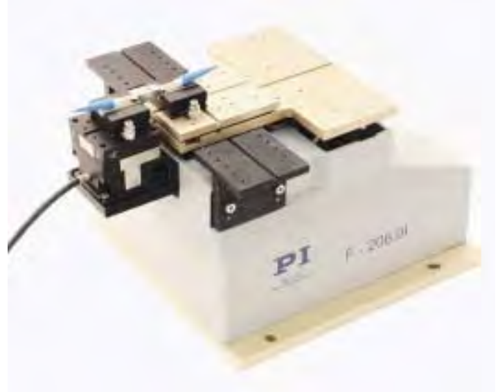
F-206 HexAlign™ 6D alignment robot combines long-travel, high-precision, six-degree-of-freedom motion and linear/rotary alignment automation. Optional high-speed 100x100x100 \mu m, XYZ PZT scanning & alignment module achieves nanometer resolution (see P-611, p. 8-16); F-206.MHU force limiting platform (optional) protects equipment.
