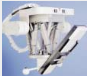
Custom Hexapod 6D robot with additional translation stage for extended travel. Application: surgery. Photo Courtesy of URS.
