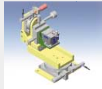
3D CAD design of a custom 5D coarse/fine fiber alignment system with closed-loop PZT drives.
