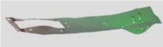
Dynamic vibration analysis of a voice-coil driven scanner measured with Polytec Laser Scanning Vibrometer
